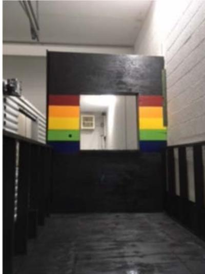
Bailout prop. Colors indicate temperatures in a fire. A reminder to stay low when bailing out.
