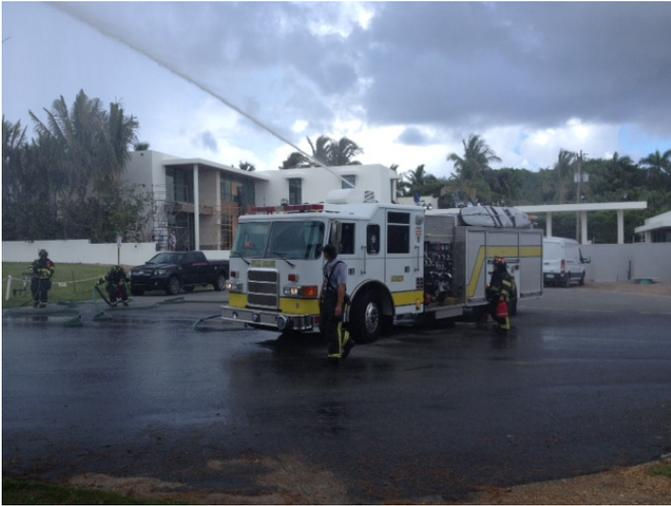
Station #2 practicing “transitional fire attack” using deckgun in conjunction with preconnect handline.
