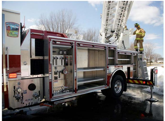
er along with two hose reels. This configuration opens up more space in the compartments while increasing the speed and efficiency for deploying lines when needed during vehicle extrication.
